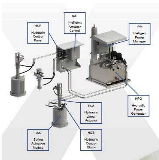
Hydraulic actuation and control system for bypass valves
